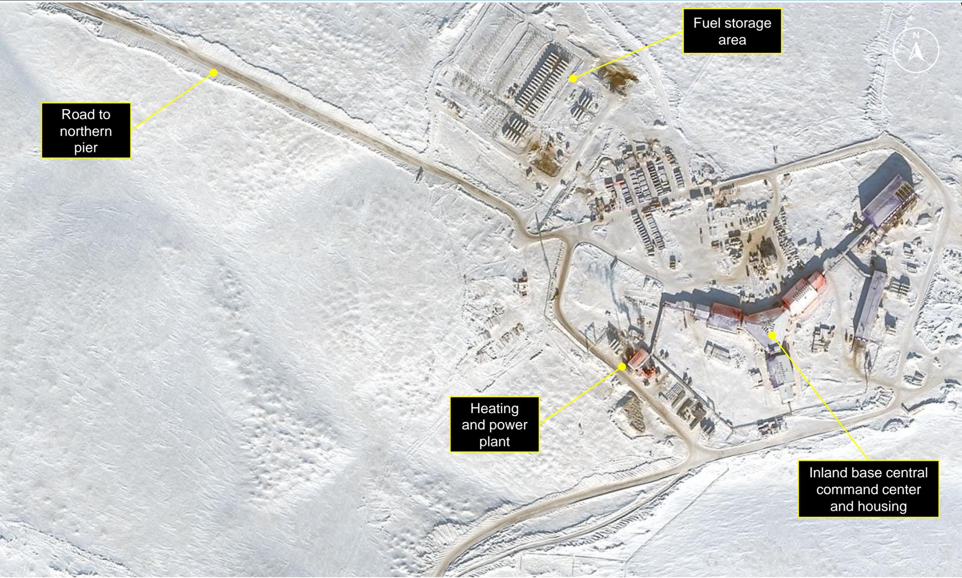
Figure 3. Temp inland base activity and construction, April 05, 2015
